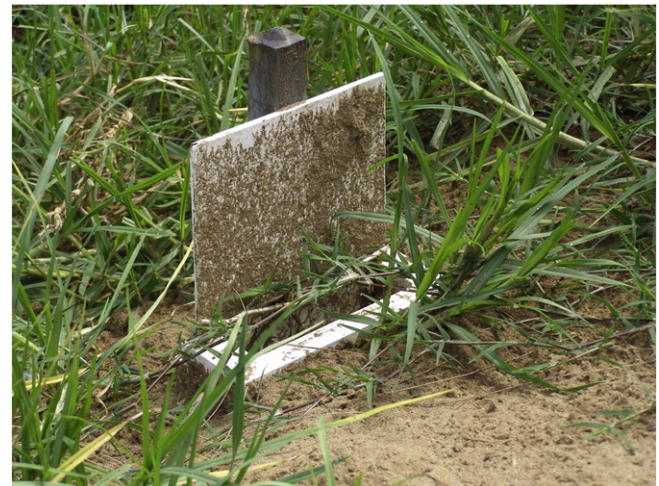
Fig. 5. Photograph of splashboard positioned at the side of a typical wombat mound. Note the accumulation of soil on the vertical face of the board following displacement during rainfall.
